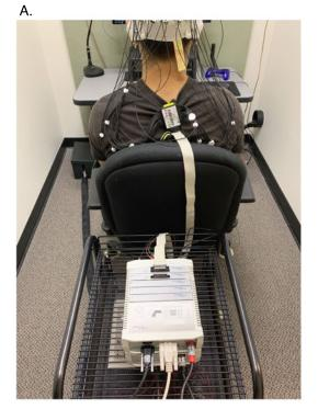
Figure 7. Illustration of optimal amplifier placement (panel A) and unstrained cables connecting the electrodes to the amplifier (panel B).
